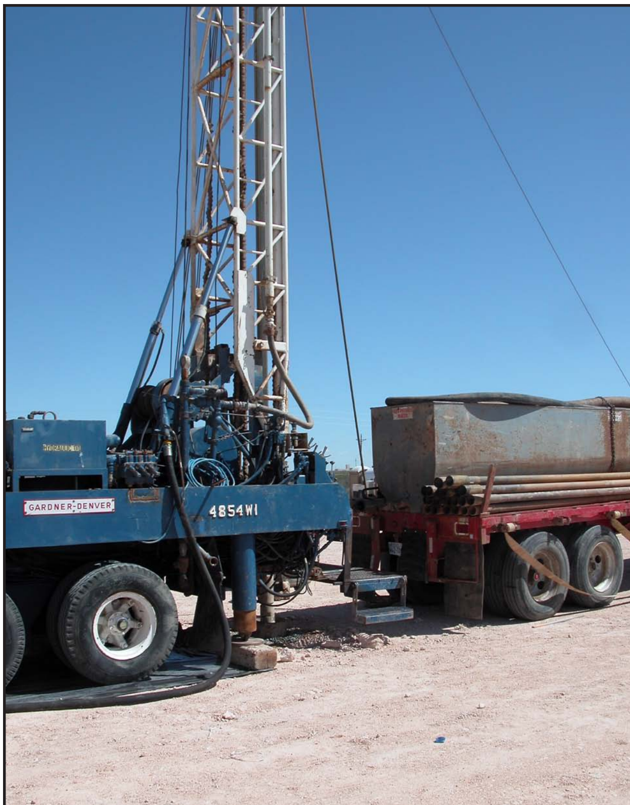
West Texas Water Well Service Rig #15 at SNL-13, viewed toward the northeast. The waste shaft at WIPP is visible between the drill rig and pipe truck. A temporary surface conductor casing is cemented in place in preparation for drilling with air. Taken April 11, 2005, by Dennis W. Powers.
