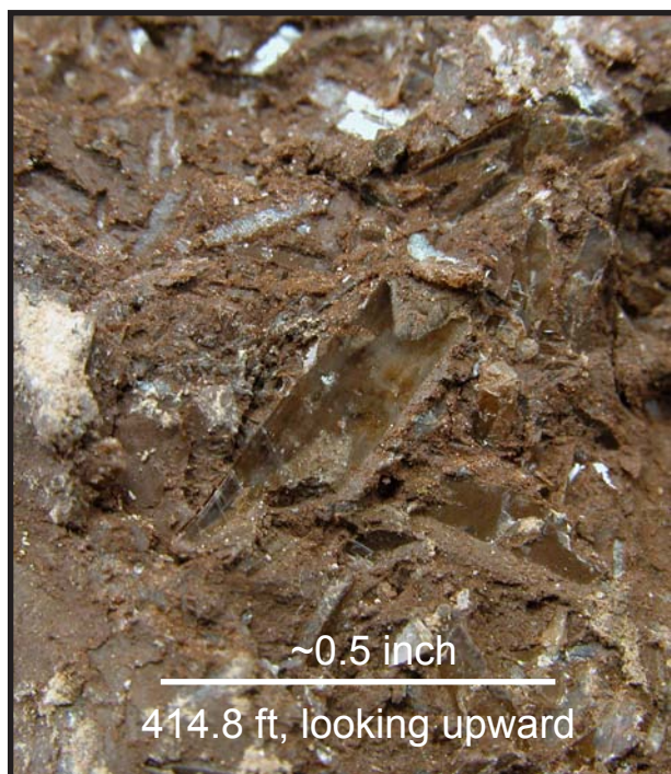
Figure 2-7. Displacive Gypsum in Reddish-Brown Siltstone From M-2.
