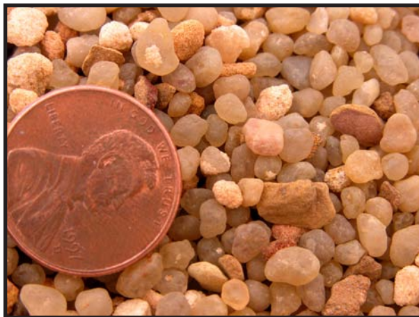
Figure 3-4. Gravel (4/10) Used to Pack Annulus Behind Screen
